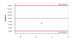
These final test values refer to the delivered nominal volume (max, volume), instrument and liquid (dist, water) at equilibrium with ambient temperature (20 °C). The test was effected according to ISO 648
