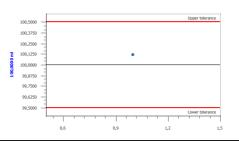
These final test values refer to the delivered nominal volume (max. volume), instrument and liquid (dist. water) at equilibrium with ambient temperature (20 °C). The test was effected according to ISO 4788
