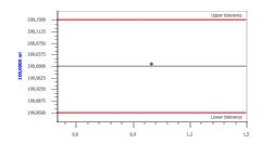
These final test values refer to the delivered nominal volume (max. volume), instrument and liquid (dist, water) at equilibrium with ambient temperature (20 °C). The test was effected according to ISO 1042
