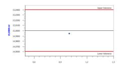
These final test values refer to the delivered nominal volume (max. volume), instrument and liquid (dist. water) at equilibrium with ambient temperature (20 °C). The test was effected according to ISO 1042
