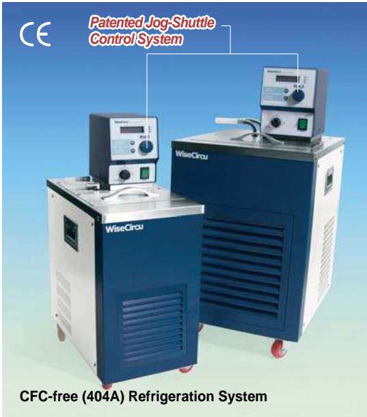
Digital Precision Refrigerated Bath Circulators (WCR-P6 & WCR-P12)
